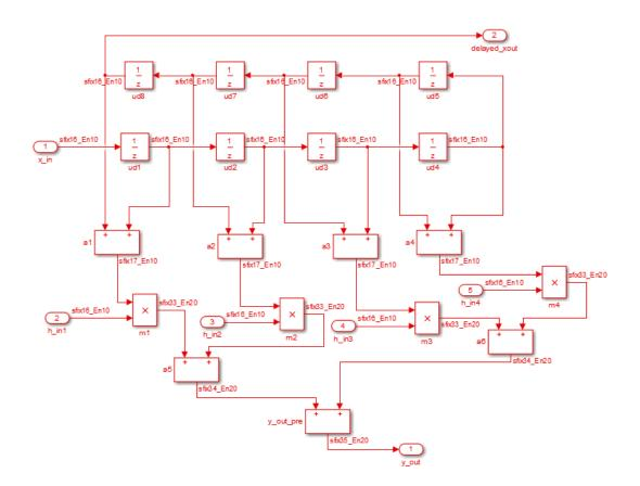
The following figure shows the symmetric\_fir subsystem.
